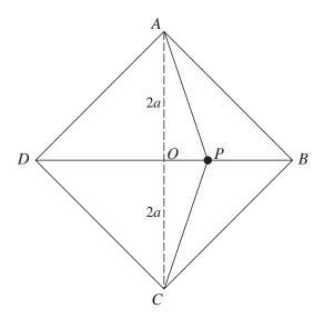
ABCD is a smooth square horizontal table with centre O and diagonals of length 4a. A particle P of mass m rests on the table and is connected to A and to C by two light elastic strings, each of natural length a and modulus of elasticity  $\lambda$  (see diagram). Show that, when P is displaced a short distance x from O towards B, the resultant force towards O is  $\frac{\lambda x}{a}$ , if  $\left(\frac{x}{a}\right)^2$  and higher powers of  $\frac{x}{a}$  are neglected. [5]
